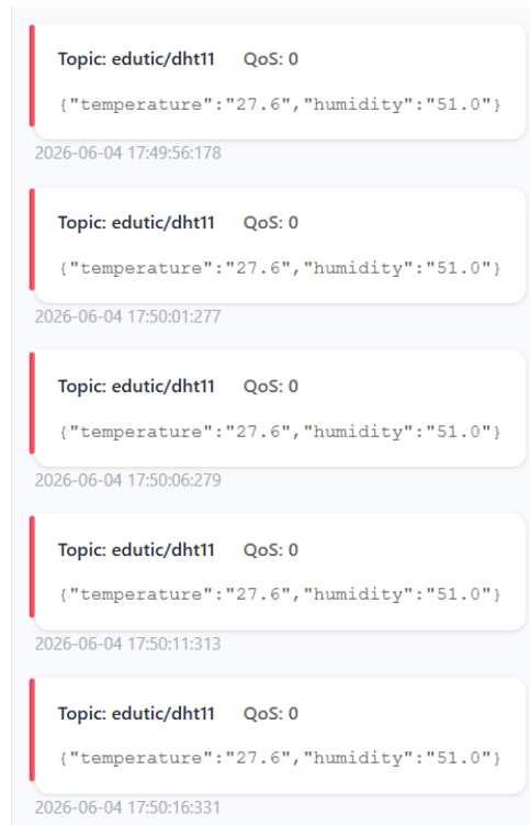
Figure 5. MQTT message transmission and reception monitoring.
